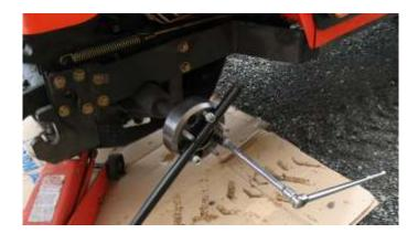
H. Reinstall the wheel & torque the nuts to 70ft. lbs for the rear wheels. We have found that having a metal shovel and rolling the tire onto it, makes the job of lining up everything must easier. One can slide the tire around, pry & lever the tire into place.
