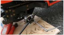
H. Get your socket & add Loctite to the studs on the spacer. Install the rim/wheel & now use the new Lock Washer & nuts from the spacer, making sure they are flip to the proper end. Torque the nuts to 110 ft. lbs for the rim in the same 3 steps as above.
