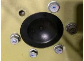
F. The factory bolts treads are 14mmx1.5 tread, We have supplied new Lug bolt 14mmx1.5 use these to install the spacer to the axle  $\triangle$ Important the OEM lug bolt are not long enough, do not reuse these.
