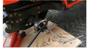
H. Get your deep socket, install the rim/wheel (using a steel Shovel, under the tire and moving it around makes it easier to get everything align) & now use the new lock washers supplied & the nuts from the spacer. Torque the nuts to 130 ft. lbs for the rim in the same 3 steps as above.
