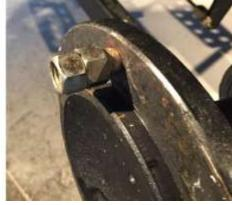
G. You will need to remove the 2 Stud on the axle, double nut tight the Stud as in photo & turn counter clockwise the inside nut. The stud should unscrew itself from the axle. We supplied new Lug Bolt (gold), add loctite to the lug bolt & install the spacer to the axle. Do not use lock washer, these are to be used on the wheel.
