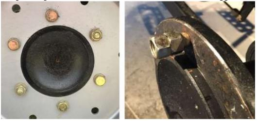
You will need to remove the 2 Stud on the axle, double nut tight the Stud as in photo & turn counter clockwise the inside nut. The stud should unscrew itself from the axle.
