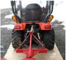
None < Spacer > With .....the tractor is way more stable...Finish pic with spacers on Wheels
