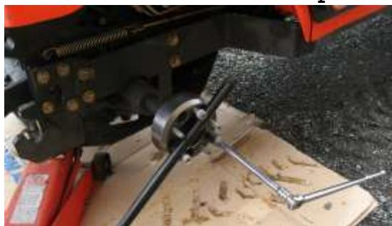
H. Reinstall the wheel & install the & torque the new gold nuts to 65 ft. lbs for the wheels.
