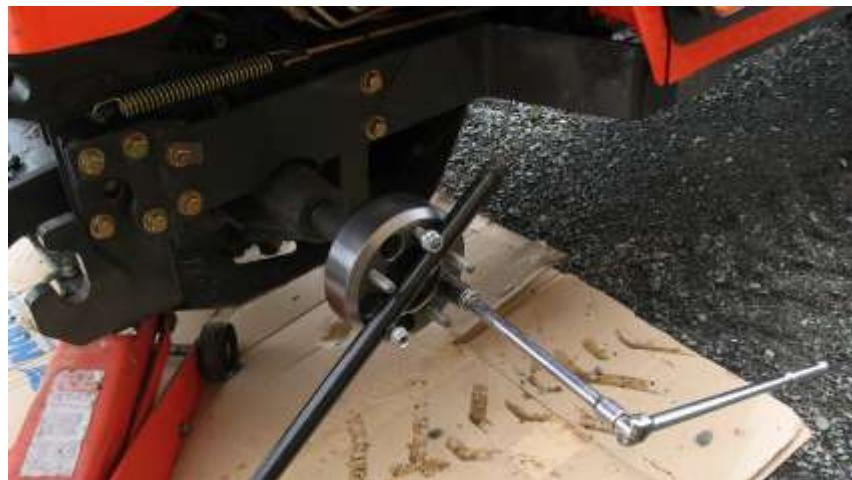
H. Reinstall the wheel & torque the nuts(if OEM had lockwasher, reused them) to 80-96 ft. lbs for the rear wheels. We have found that having a metal shovel and rolling the tire onto it, makes the job of lining up everything much easier. One can slide the tire around, pry & lever the tire into place.
