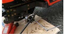
H. Reinstall the wheel & torque the nuts to 70 ft. lbs for the rear wheels.
