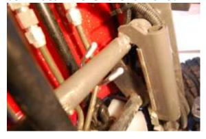
.6 Reinstall the two nylon nuts & washers on the u-Bolt andtightening only, this leave some play that will make it easier to line up the skid plate.
