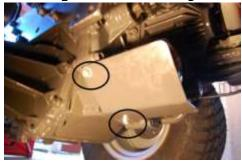
Remove the two rear bolts at the back of the 3 point hitch. These shall be reuse in step .4
