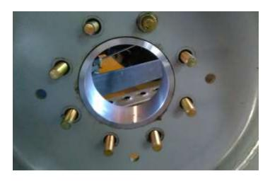
I. Check clearances around the Wheel, no point of contact should be noticed.
