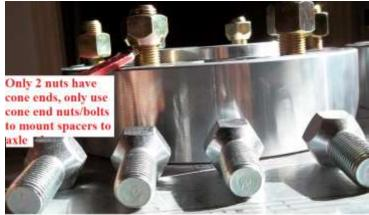
$\triangle$ Please take the time to make the install in 3 steps. First hand tightens the bolts; Second torque the bolts to half the torque in a crisscross pattern & finally torque the bolt to their final value of 150 ft-lb for the rear's wheels.
