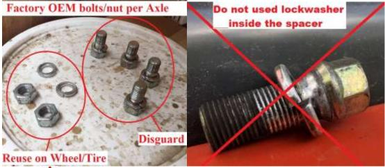
⚠ do not mix these up. You should now have 2 factory nuts/lock washer. Disregard the 4 factory bolts/lock washer. We supplied new Lock Washer for the install of the wheel. In Step "H" to install the rim
