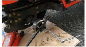
H. Reinstall the wheel & install the & Torque the new gold nuts to 70 ft. lbs for the rear wheels.
