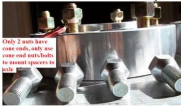
$\Delta$ Please take the time to make the install in 3 steps. First hand tightens the bolts; Second torque the bolts to half the torque in a crisscross pattern & finally torque the bolt to their final value of 150 ft-lb for the rear's wheels.
