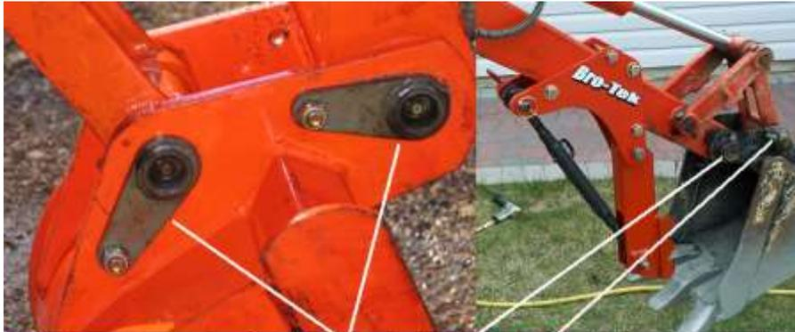
BX24 has a new setup for the pins, the BX22 & BX23 pins have one hole drill at one end, which a bolt holds the pin in place.
