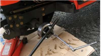
H. Get your socket & add Loctite to the studs on the spacer. Install the rim/wheel & now use the new nuts from the spacer, making sure they are flip to the proper end. Torque the nuts to 110 ft. lbs for the rim in the same 3 steps as above.
