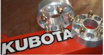
G.To install the spacers, you will need a long bar to hold the axle from turning, add Blue Thread locker to the bolts.
