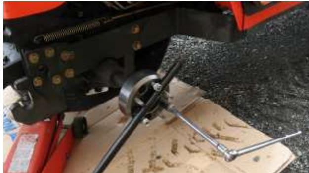
H. Get your socket & add Loctite to the studs on the spacer. Install the rim/wheel & now use the new nuts from the spacer, making sure they are flip to the proper end. Torque the nuts to 90 ft. lbs for the rim in the same 3 steps as above (3/4" Socket).
