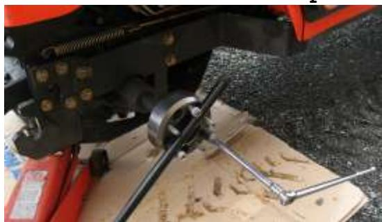
H. Reinstall the wheel & install the & torque the new gold nuts to 65 ft. lbs for the rear wheels.
