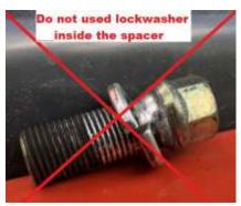
△ do not mix these up. You should now have 2 factory nuts/lock washer. Disregard the 4 factory bolts/lock washer. We supplied new Lock Washer for the install of the wheel. In Step "H" to install the rim
