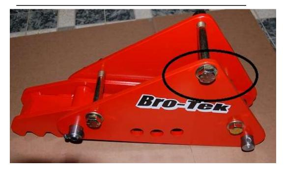
D. Install other two bolts, in the lower holes. Do not tighten them all the way.
