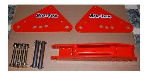
For the first time around, install the top two bolts (some thumbs only require 1), Lock nut & Washer. Do not tight it all the way, like the one in photo.
