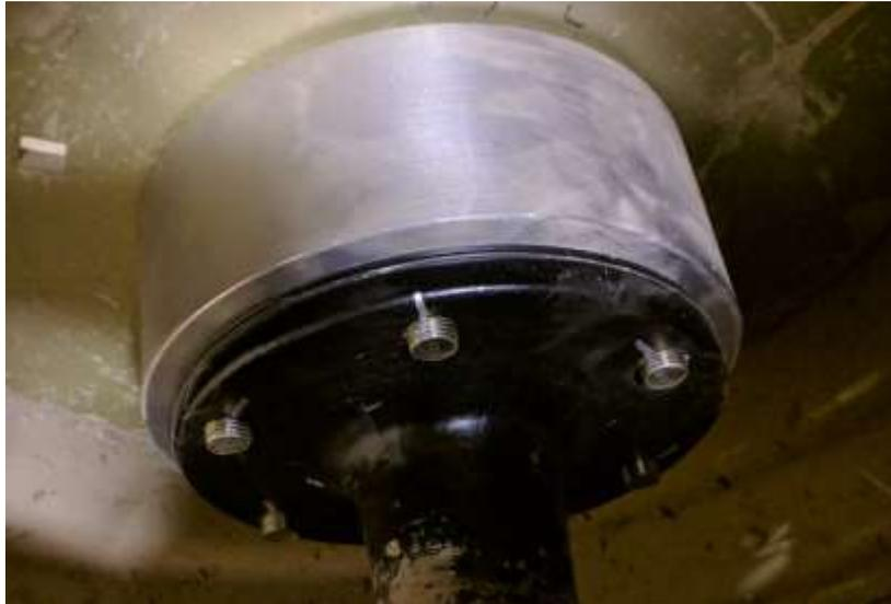
Using the "Paint pen" leave a line going from the backside of the axle flange onto the end of the tread lug bolts. Do the same on the outside of the wheel side. This way if the lug bolts break themselves lose, the paint line will no longer align, warning you of needing retorque everything up.
