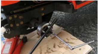
Please take the time to make the install in a 3 steps. First hand tighten the Lug bolts (new gold we supplied); Second torque the bolts to half the torque in a crisscross pattern & Finally torque the bolt to their final value of 120 ft. lbs.
