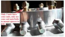
$\triangle$ Please take the time to make the install in 3 steps. <u>First</u> hand tightens the bolts; <u>Second</u> torque the bolts to half the torque in a crisscross pattern & <u>finally</u> torque the bolt to their final value of 150 lb-ft for the rear's wheels.
