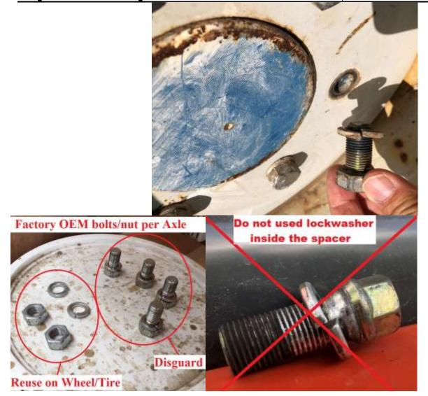
A do not mix these up. You should now have factory nuts/lock washer. Disregard the factory bolts/lock washer. We supplied new Lock Washer for the install of the wheel. In Step "H" to install the rim
