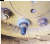
Now is a good time to test fit the spacer to the Axle & then to the wheel rim. The spacer should make full contact to the axle, the rim hole may have to be file/clean a very small amount to clear the spacer lug. It's much easier to sort any problems without having anything bolted down. If everything looks good it's time to start the install.
