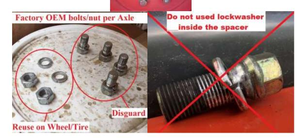
△ do not mix these up. You should now have 2 factory nuts/lock washer. Disregard the 4 factory bolts/lock washer. We supplied new Lock Washer for the install of the wheel. In Step "H" to install the rim  $\triangle$  Do not use the OEM factory bolts or nuts to install the spacer to the axle. We supplied 4 New Gold taper lug Bolts per side & take from the spacer 2 of the 6 new gold Nuts from the spacer.
