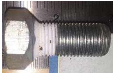
Now is a good time to test fit the spacer to the Axle & then to the wheel rim. The spacer should make full contact to the axle & the nuts/lug bolt has full tread contact
