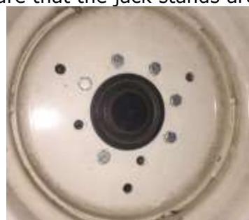
F. The factory Lug bolts treads are 9/16 tread, Reuse the OEM Lug bolt these to install the spacer to the axle
