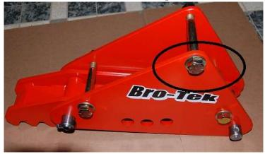
D. Install other two bolts, in the lower holes. Do not tighten them all the way.
