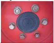
Factory OEM bolts/nut per Axle Do not used lockwasher inside the spacer Disguard Reuse on Wheel/Tire
