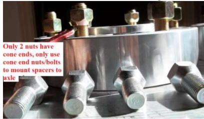
$\triangle$ Please take the time to make the install in 3 steps. First hand tightens the bolts; Second torque the bolts to half the torque in a crisscross pattern & finally torque the bolt to their final value of 150 ft. lbs for the rears wheels.
