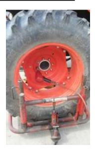
I. Check clearances around the Wheel, no point of contact should be noticed.
