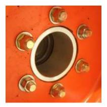
We have found that having a metal shovel and rolling the tire onto it, makes the job of lining up everything must easier. One can slide the tire around, pry & lever the tire into place.
