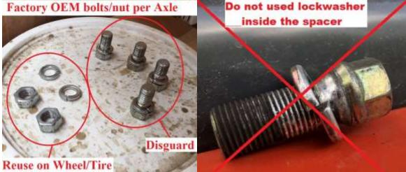
A do not mix these up. You should now have 2 factory nuts/lock washer. Disregard the 4 factory bolts/lock washer. We supplied new Lock Washer for the install of the wheel. In Step "H" to install the rim  $\triangle$  Do not use the OEM factory bolts or nuts to install the spacer to the axle. We supplied 4 New Gold taper lug Bolts per side & take from the spacer 2 of the 6 new gold Nuts from the spacer.
