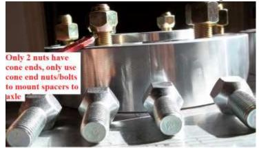
Please take the time to make the install in a 3 steps. <u>First</u> hand tightens the bolts; <u>Second</u> torque the bolts to half the torque in a crisscross pattern & <u>Finally</u> torque the bolt to their final value of 150 ft. lbs for the rears wheels. <u>A new Gold Lug bolt & 2 new Nut from</u>
