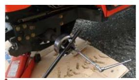
First add the Loctite & hand tighten the new Lug nuts (gold lug nut we supplied, which are on the spacers); Second torque the nut to half the torque in a crisscross pattern & Finally torque the bolt to their final value of 120 ft. lbs.
