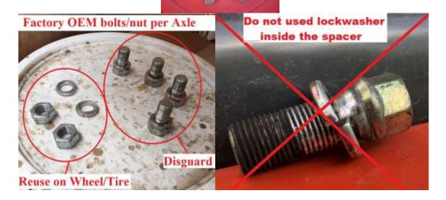
do not mix these up. You should now have 2 factory nuts/lock washer. Disregard the 4 factory bolts/lock washer. We supplied new Lock Washer for the install of the wheel. In Step "H" to install the rim
