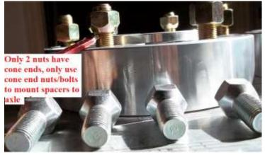
$\Delta$ Please take the time to make the install in a 3 steps. First hand tightens the bolts; Second torque the bolts to half the torque in a crisscross pattern & Finally torque the bolt to their final value of 150 ft. lbs for the rears wheels.
