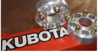
G.To install the spacers, you will need a long bar to hold the axle from turning, add Blue Thread locker to the bolts.
