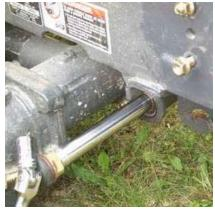
Take one of the 3/8" plate and use one of our supplied bolts, which are longer than the OEM. Put Loctite on & use the Top bolt first, the nut is pre welded behind the frame. Photo below is looking up, from under the frame.
