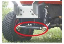
The guard is built to accept the factory OEM Top-link, which comes with the tractor 3-point kit, using 4''-34'' pins & clips. Our Tool box will also bolt-on, instead of the Top-link, to act as a sacrifice piece. Tool box is great to carry chains, tools or Top-link.
