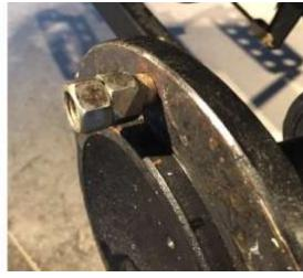
F. The factory axle lug Nut are the same tread type (M18x1.5) but not the same cone spacer as the supplied gold Nut, which are cone/taper to be used inside the spacer. (Make sure to save the factory lock washer (on the wheel side) but the factory nut & lug bolt, will not the reused. Only the supplied gold lug bolt goes inside the spacer; butno lockwasher at this step).
