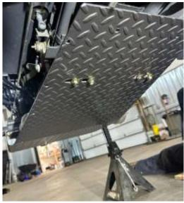
.7 Torque the nuts (1/2" wrench) on the U-Bolt to 10 lb.-ft and 65 lb.-ft the 2-rear bolt on the axle casting.
