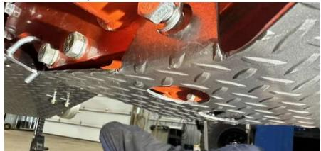
.4 Install the last U-Bolt all the way to the front around the front axle tube & line everything up before torquing down (photo below).
