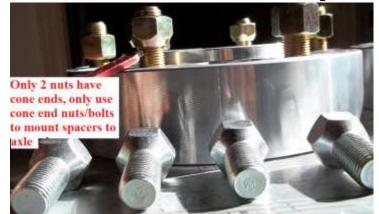
A Taper ends must make contact with the spacers.
