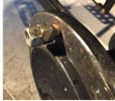
G. You will need to remove the 2 Stud on the axle, double nut tight the Stud as in photo & turn counter clockwise the inside nut. The stud should unscrew itself from the axle. We supplied new Lug Bolt (gold), add loctite to the lug bolt & install the spacer to the axle. Do not use lock washer, these are to be used on the wheel.
